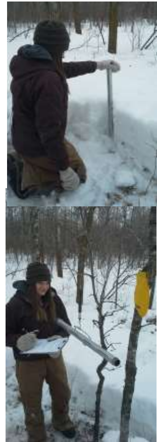
Establishing weight of snow sample to calculate water content
